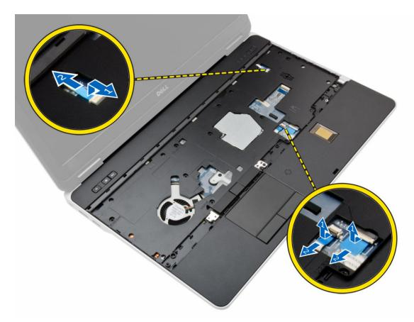
6. Pry the palmrest assembly upwards and remove it from the computer.
