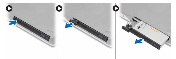
**4.** Remove the screw that secures the optical-drive latch to the optical drive. Slide the optical-drive latch and remove it from the optical-drive.
