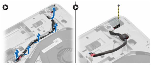
4. Lift the power-connector bracket from the computer. Lift the power connector from the computer.
