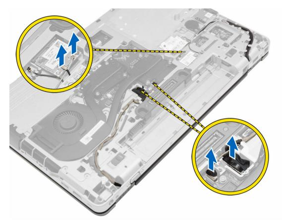
4. Disconnect the LVDS cable and release the LVDS cable and camera cable from the routing channel. Remove them from the computer.
