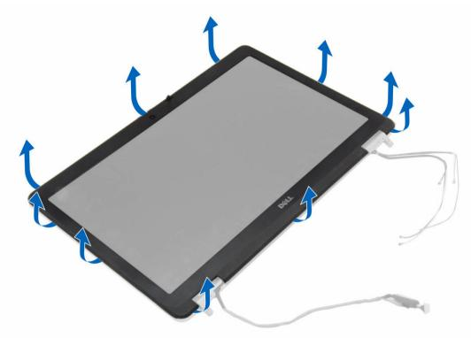
4. Remove the display bezel from the display assembly.
