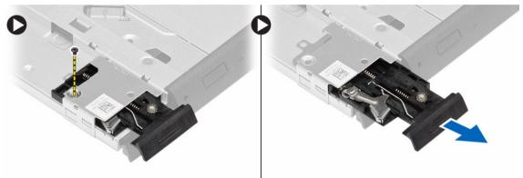
5. Remove the screws that secure the optical-drive latch bracket to the optical drive. Remove the latch bracket from the optical drive.
