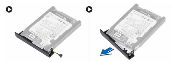
5. Flex the hard-drive isolation. Peel off the hard-drive isolation from the hard drive.
