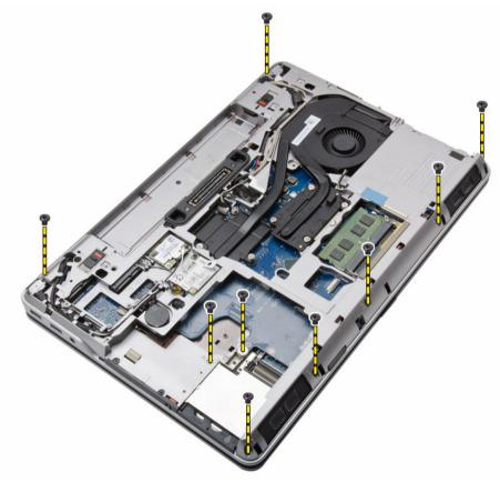
4. Flip the computer and remove the screws that secure the palmrest assembly to the computer.
