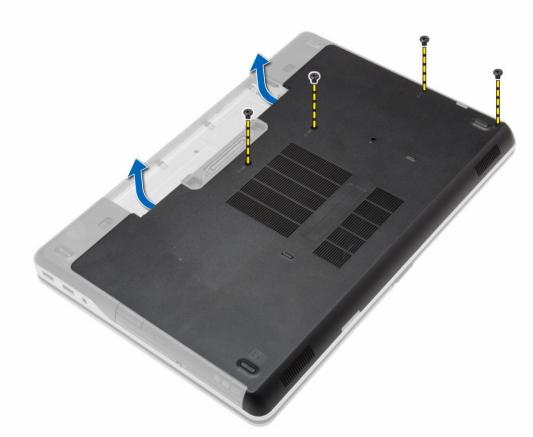
4. Lift the base cover and remove it from the computer.
