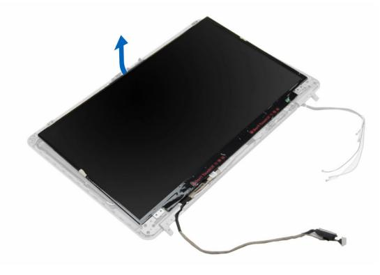
5. Peel off the LVDS cable-connector tape and disconnect the LVDS cable from the display panel. Remove the display panel from the display assembly.
