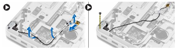
4. Lift the network-connector bracket from the computer. Lift the network connector from the computer.
